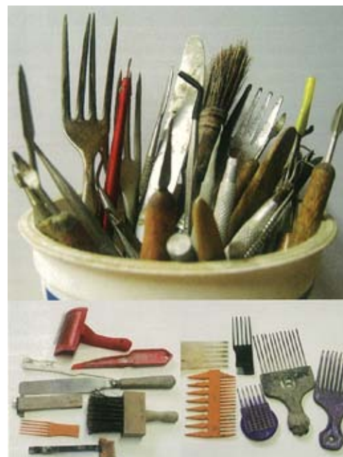
FIG. 116 Divers outils de modelage permettant de texturer la surface du ciment (D. Tucker).
